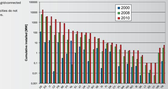
**Fig. 4:** Cumulative installed grid-connected PV capacity in EU + CC Note that the installed capacities do not correlate with solar resources.
